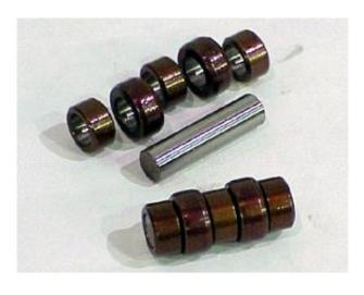
Remove the roller and axle assemblies and set on a clean surface until re-assembly.
