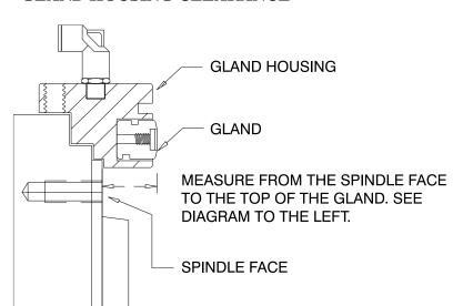
While putting on the Gland Housing be sure to measure for clearance between the chuck and Gland Housing. This distance should be .030" to .040" less than the length from the back of the chuck to where the gland seals. See Illustration below. This will allow clearance for the chuck to rotate freely.
