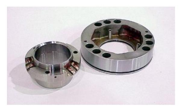
Remove the  $\frac{1}{4}$ -20 x 2-1/2" screws from the piston. Remove the ramp from the piston.
