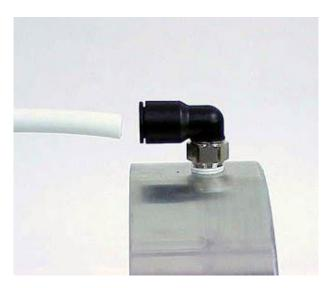
Connect air supply from the valve to the gland housing using the  $\frac{1}{2}$ " airline supplied with the kit. The port in the gland housing is tapped  $\frac{3}{8}$  –  $\frac{18}{18}$  NPT. Cut off any excess airline and tie up loose or drooping line with wire ties.
