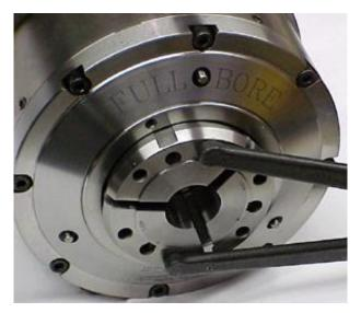
The chuck may release the workpiece due to low grip force. With the pins above flush, the collet grip force drops significantly. Remember, when the pins are extended out all the way, the collet is open and the workpiece is released.
