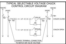
Locate the terminal strip in the electrical cabinet that has the connections for the Chuck Open and Chuck Close solenoids. Locate an area on the electrical cabinet near this terminal strip for the air valves' power cord to enter the cabinet. Drill a pilot hole and use a ½ chassis punch to punch out a hole for the cord grip.
