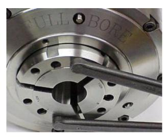
Clamping force or grip force is adjusted by screwing the collet in or out of the chuck. Grip force is increased by the clockwise rotation of the collet. Maximum clamping force is achieved when the indicator pins are flush with the counterbores in the faceplate. To reduce the grip force, rotate the collet counterclockwise until the desired grip is attained. With the force less than maximum, the indicator pins will sit at a position below flush with the counterbores.
